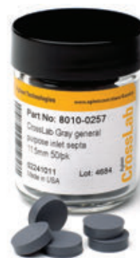
CrossLab general purpose inlet septa, 8010-0257
